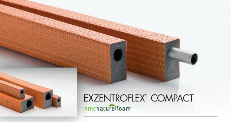
Exzentroflex® COMPACT is an excentric polyethylene-based, closed-cell foam pipe insulation, made of NMC Naturefoam® which contains at least 50% of renewable raw materials, with a robust shell for insulation of heater connecter pipes in flooring.
