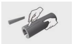
...and glue the joints of the cut surfaces together, to reduce the diameter of the tube end.
