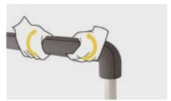
Seal all joints with NMC-fix glue. Do not stretch when sealing joints.
