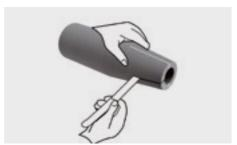
Then glue the joints together, also the tube ends with the insulation of the pipes.
