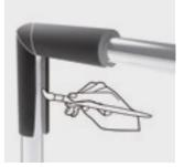
...cautiously cut the elbow piece along its throat. Fit the insulation elbow on the pipe and apply glue on the edges. You may apply the glue on the joints before or after placing the elbow on the pipework. Press the joints together to seal. Carefully glue the joints of the elbow and of the straight tube positioned on either side.
