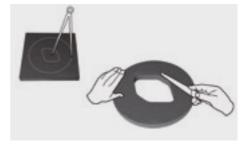
Position the disc and stick the edges together with NMC-fix glue. Make sure to stick the inside edges to the face plate, too.
