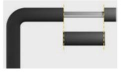
Cut the insert in the length and seal the edges. Consider to glue all the joints properly.
