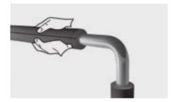
Push in rotatory motions the INSUL-TUBE  $\ensuremath{^{\circ}}$  tube along the pipe
