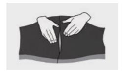
Wrap the INSUL ROLL insulation around the pipe and press the joints tightly together.
