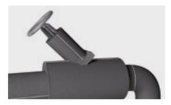
Cut out a ring of INSUL ROLL sheet in the size of the stopcock wheel. The inner diameter should be the same as the outer diameter of the sleeve already attached.
