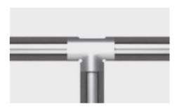
Make a Tee-cover as earlier described. However, use a tube with an internal diameter equal to the external diameter of the neighbouring tubes.
