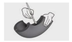
Wrap the INSUL ROLL insulation around the pipe and press the joints tightly together.
