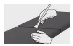
Similarly, to the insulation of tanks with normal INSUL ROLL sheets, an insulation with self-adhesive sheets can be done.
