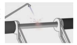
When filling in a gap between two tubes, cut the insert a little longer than necessary (a couple of millimetres) to ensure that there is enough compression and avoid a reduction of insulation properties
