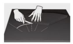
Glue the edges with NMC-Fix glue and fit the insulation, after drying to the reducer. Press the two edges together starting at the far ends.
