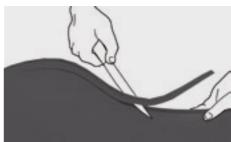
Attach the insulation material around the ring and adhere with NMC-fix glue the connecting surfaces together.
