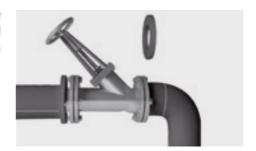
Measure the distance between the two INSUL ROLL rings, including the material itself, and the distance between each ring and the stopcock housing.
