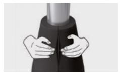
Glue the upper and lower edges with NMC-Fix glue and attach the other INSUL ROLL sections.
