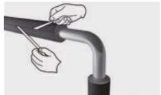
Close the slit and press firmly the joints together in order to ensure a permanent seal.
