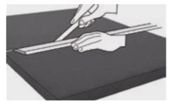
Mount the sleeve section around the rings and adhere all edges.
