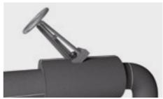
Insulate the stopcock mechanism using a cut-out of an INSUL ROLL sheet.
