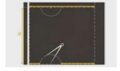
Cut out the piece, wrap it around the rings to seal the central housing, and then stick the edges together using NMC-fix glue.
