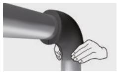
Ensure the insulation butts precisely up against the tubing to be fitted on either side.
