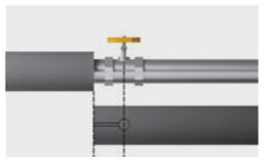
Fit the tube tightly around the valve and glue the joints together, then attach it to the adjacent tube.
