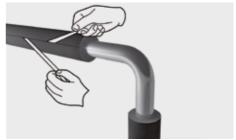
Close the slit and press firmly the joints together in order to ensure a permanent seal.
