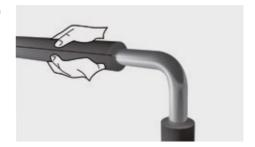
Push in rotatory motions the AEROFLEX  $\!\!\!^{\circ}$  tube along the pipe.
