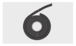
Cut out an AEROFLEX $^{\otimes}$  ROLL sheet to the size required.
