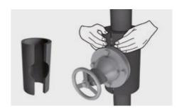
Next, calculate the shape of the disc for the front flange. Measure the circumference of the supporting flange and the form of the face flange around which the disc must fit.
