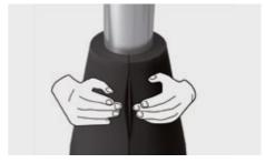
Glue the upper and lower edges with AEROSEAL glue and attach the other AEROFLEX® ROLL sections.
