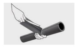
Place the cover on the Tee-connection. Apply the glue if not already done. Consider the flash-off time. Press firmly the joints together.
