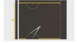
Cut out the piece, wrap it around the rings to seal the central housing, and then stick the edges together using AEROSEAL glue.
