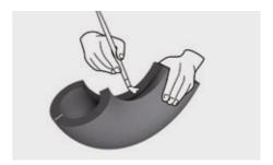
Wrap the AEROFLEX® ROLL insulation around the pipe and press the joints tightly together.
