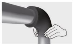
Ensure the insulation butts precisely up against the tubing to be fitted on either side.
