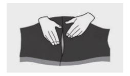
Wrap the AEROFLEX® ROLL insulation around the pipe and press the joints tightly together.
