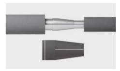
Cut the cover piece lengthwise and place it on the pipe connection.
