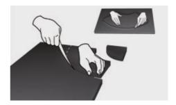
Holding the two sections together with the smooth surface on the outside, apply AEROSEAL glue to the outer edges.
