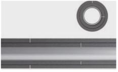
Seal all butt joints with AEROSEAL glue.
