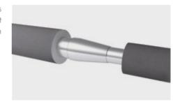
Take a piece of AEROFLEX® tube with the same diameter as the larger one of the already insulated tubes.
