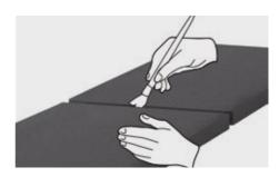
Similarly, to the insulation of tanks with normal AEROFLEX® ROLL sheets, an insulation with self-adhesive sheets can be done.
