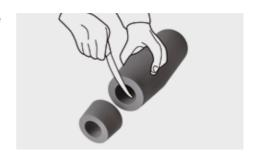
Shorten the other end too, so that the connection piece fits properly into the gap between the two insulated pipes.
