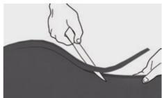
Attach the insulation material around the ring and adhere with AEROSEAL glue the connecting surfaces together.
