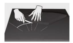
Glue the edges with AEROSEAL glue and fit the insulation, after drying to the reducer. Press the two edges together starting at the far ends.
