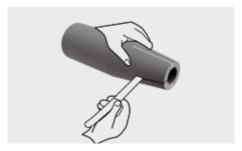
Then glue the joints together, also the tube ends with the insulation of the pipes.
