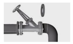
Measure the distance between the two AEROFLEX® ROLL rings, including the material itself, and the distance between each ring and the stopcock housing.
