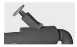
Cut out a ring of AEROFLEX® ROLL sheet in the size of the stopcock wheel. The inner diameter should be the same as the outer diameter of the sleeve already attached.
