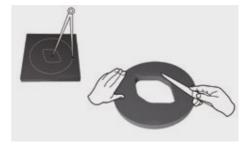
Position the disc and stick the edges together with AEROSEAL glue. Make sure to stick the inside edges to the face plate, too.
