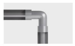
Then take an AEROFLEX® tube with an inner diameter equal to the outer diameter of the smaller tubes already installed on either side.
