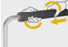
**Please note:** If the insulation is subject to compression and as a result, there is strain on the glued joints, segmented bends have be cut.
