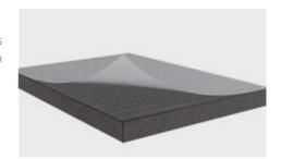
Line the edge up and stick it down. Pull the backing paper off gradually, pressing the material down as you go.
