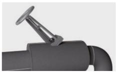
Insulate the stopcock mechanism using a cut-out of an AEROFLEX® ROLL sheet.
